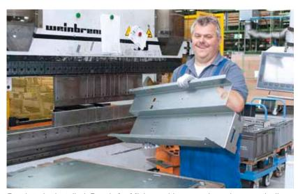
Ready to be installed: Panels for Miele machines are shaped automatically before they are fitted by the members of staff.
